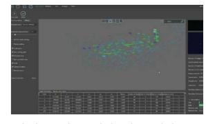
Glopho stitches coded and uncoded targets taken in the photos and optimizes the data.
