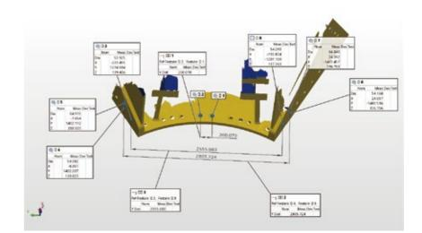
The probe locations can be approached from any angle as long as the i-Probe is within the optical tracker cameras' field of view. i-Probe's poses can be tracked and mapped to the coordinate systems in real time by the tracker so that it can measure continuously without the need to reposition.
